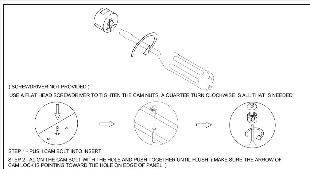
STEP 3 - THE HEAD OF THE BOLT GOES INTO THE WIDE MOUTH OF THE CAM LOCK.YOU THEN TURN THE LOCK SO THE NARROW PART CLOSES OVER THE BOLT.
