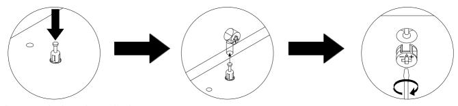
STEP 1 - PUSH CAM BOLT INTO INSERT
