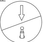
STEP 1 - PUSH CAM BOLT INTO INSERT
