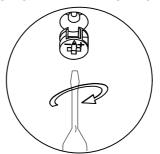
STEP 3 - THE HEAD OF THE BOLT GOES INTO THE WIDE MOUTH OF THE CAM LOCK. YOU THEN TURN THE LOCK SO THE NARROW PART CLOSES OVER THE BOLT.
