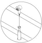
STEP 2 - ALIGN THE CAM BOLT WITH THE HOLE AND PUSH TOGETHER UNTIL FLUSH. ( MAKE SURE THE ARROW OF CAM LOCK IS POINTING TOWARD THE HOLE ON EDGE OF PANEL. )
