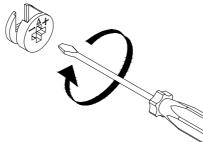
(SCREWDRIVER NOT PROVIDED) USE A FLAT HEAD SCREWDRIVER TO TIGHTEN THE CAM NUTS. A QUARTER TURN CLOCKWISE IS ALL THAT IS NEEDED.
