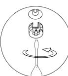
STEP 1 - PUSH CAM BOLT INTO INSERT
