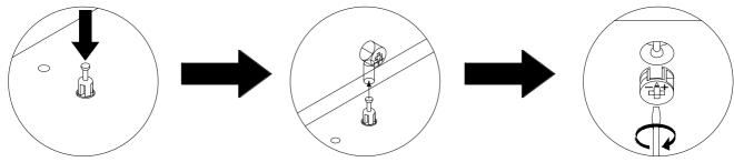
STEP 1 - PUSH CAM BOLT INTO INSERT
