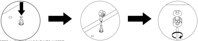
STEP 1 - PUSH CAM BOLT INTO INSERT
