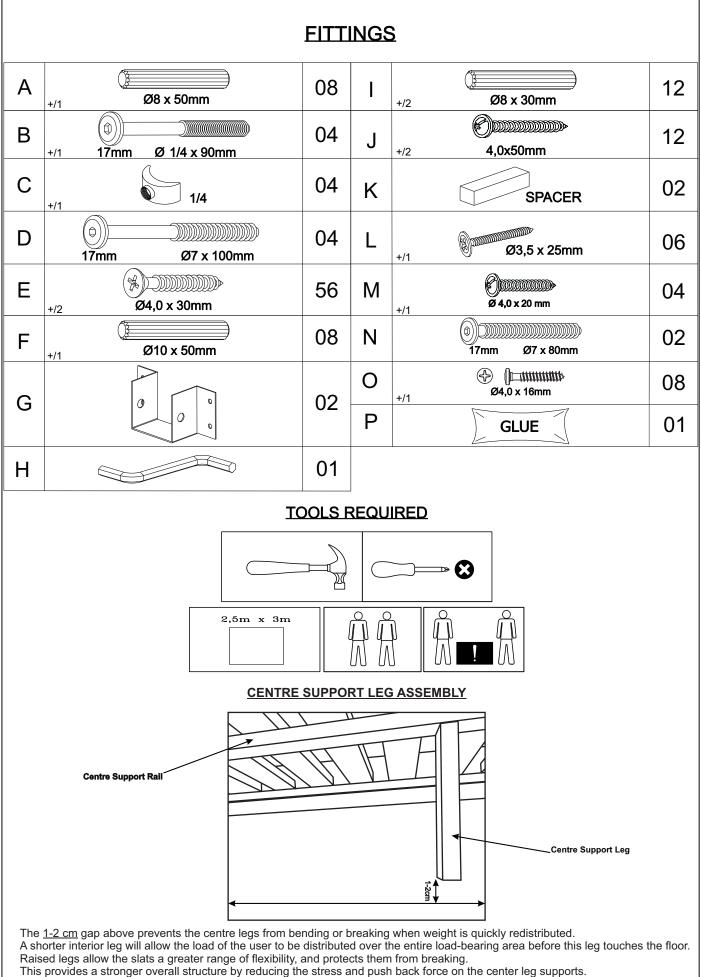
If the bed is moved or repositioned, interior legs cannot be dragged and are safeguarded from damage.
