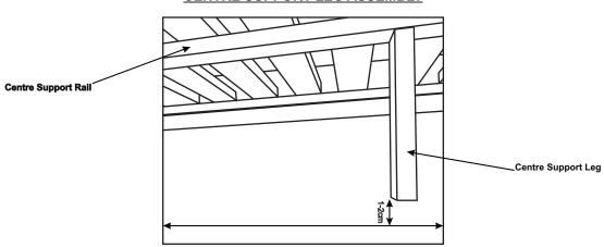
The 1-2 cm gap above prevents the centre legs from bending or breaking when weight is quickly redistributed. A shorter interior leg will allow the load of the user to be distributed over the entire load-bearing area before this leg touches the floor. Raised legs allow the slats a greater range of flexibility, and protects them from breaking.
