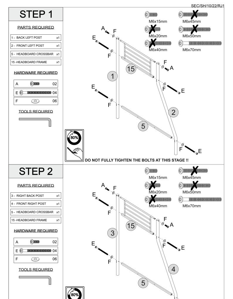
DO NOT FULLY TIGHTEN THE BOLTS AT THIS STAGE!!
