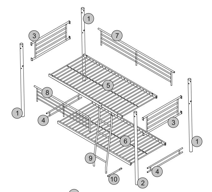
PLEASE NOTE: UPPER BASE (5) HAS HOLES FOR ASSEMBLY OF LADDER AND SAFETY RAILS
