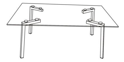
THIS PRODUCT INCLUDES TOUGHENED GLASS WITH A NOMINAL THICKNESS OF 8MM. IF THE GLASS IS CHIPPED OR BROKEN, PLEASE REPLACE WITH TYPE DESCRIBED OR ALTERNATIVELY CONSULT WITH THE RETAILER STATING THE MODEL DETAILS.
