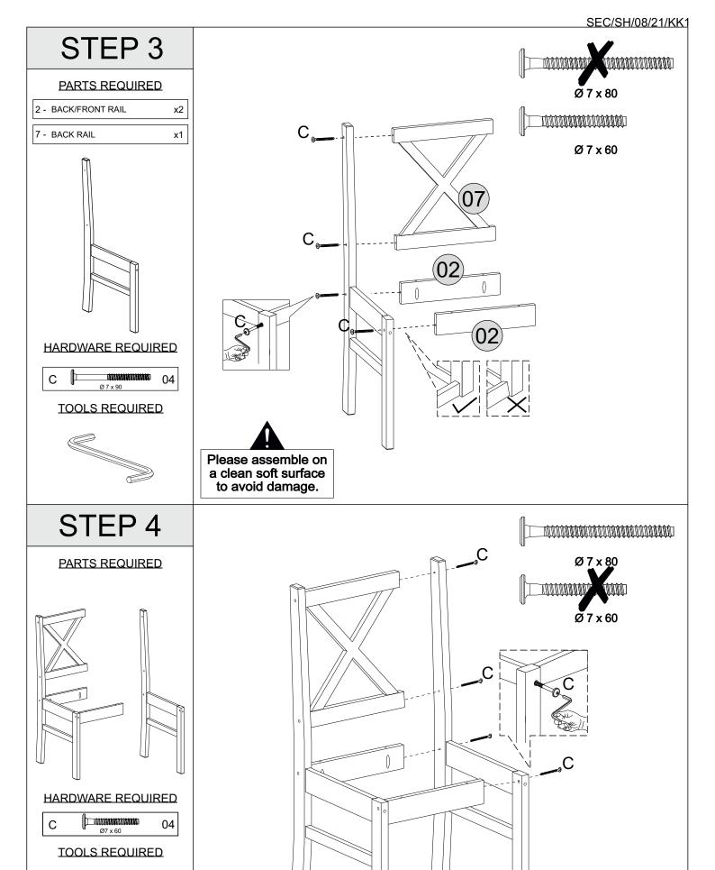
Please assemble on a clean soft surface to avoid damage.
