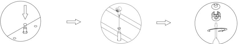
STEP 1 - PUSH CAM BOLT INTO INSERT
