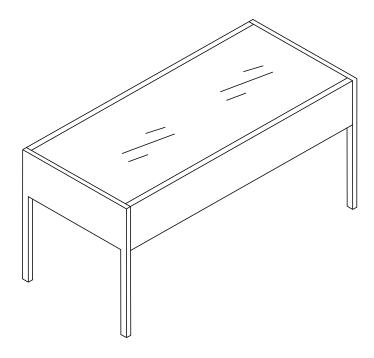
THIS PRODUCT INCLUDES TOUGHENED GLASS WITH A NOMINAL THICKNESS OF 5MM. IF THE GLASS IS CHIPPED OR BROKEN PLEASE REPLACE WITH TYPE DESCRIBED OR ALTERNATIVELY CONSULT WITH THE RETAILER STATING THE MODEL DETAILS.
